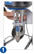
Remove rod coupling, inlet hose and paint hose
